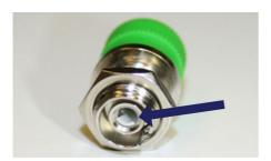
Fig. 4.8 Broken ferrule on the adapter
