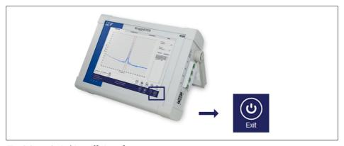
Fig. 3.3 Switching off via software
