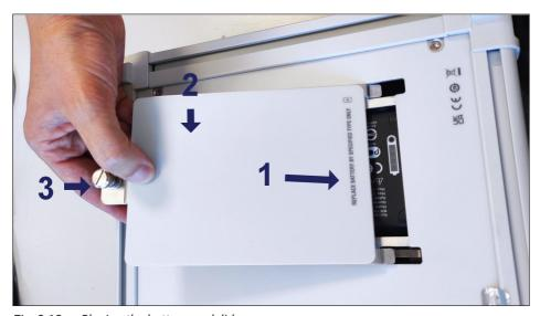
Fig. 3.12 Closing the battery pack lid
