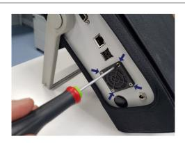
Fig. 3.15 Fan filter fixation
