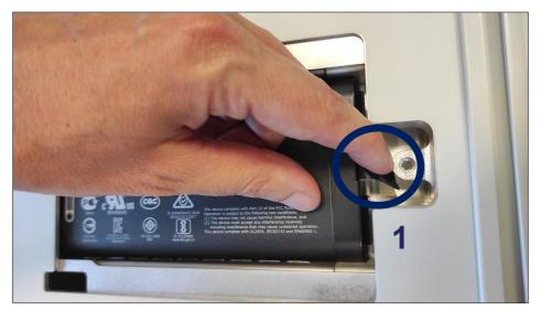
Fig. 3.11 Positioning the pull-out flap
