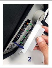
Fig. 3.17 Detachable connector panel
