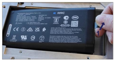
Fig. 3.9 Removing the battery pack
