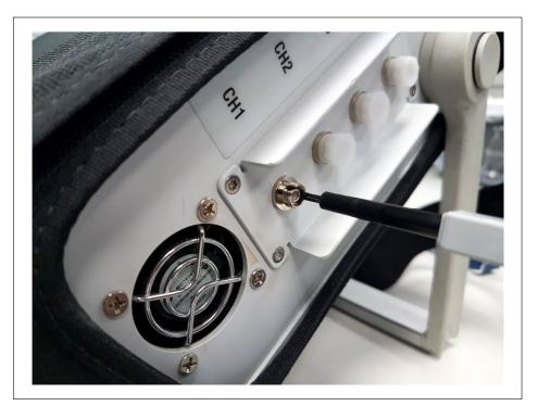
Fig. 4.7 Cleaning the adapter
