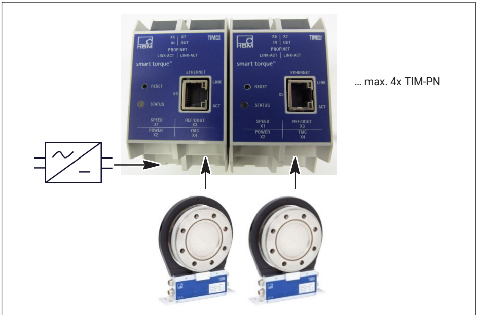
Fig. 7.1 Operating multiple TIM-PN modules connected in series
