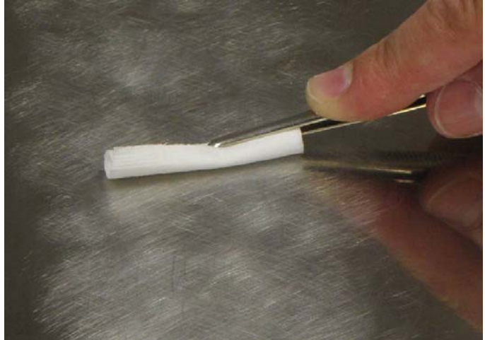
Fig. 1.4 Cleaning of roughened surface.
