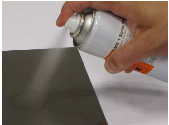
Fig. 1.1 Spraying 1-RMS on specimen
