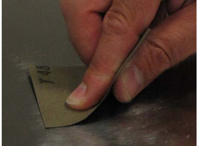
Fig. 1.3 Removal of larger impurities using emery cloth.
