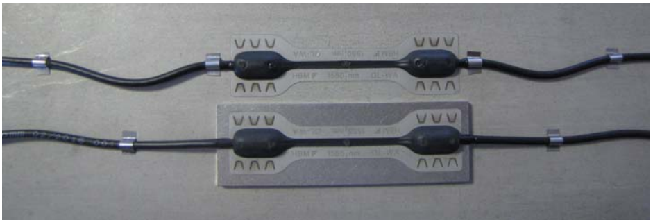
Fig. 3.1 Temperature-compensated strain measuring point with strain relief of the fiber cables
