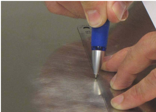
Fig. 2.6 Marking the marking lines
