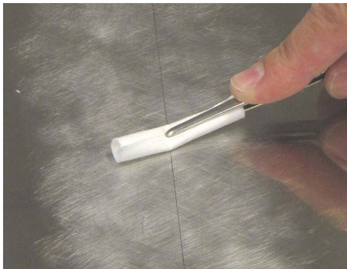
Fig. 2.7 Final cleaning of the installation point
