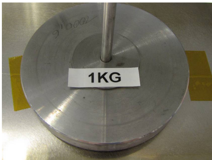
Fig. 2.11 Load on top of the optical fiber FBG bonding area
