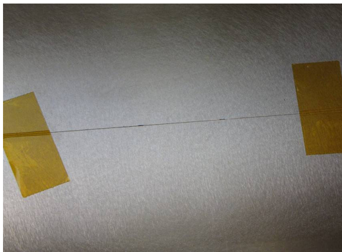
Fig. 2.8 Fixing the optical fiber
