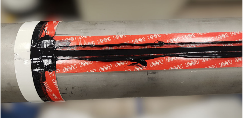
Fig. 2.21 Spreading the glue with a spatula.
