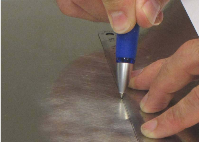
Fig. 2.6 Marking the marking lines
