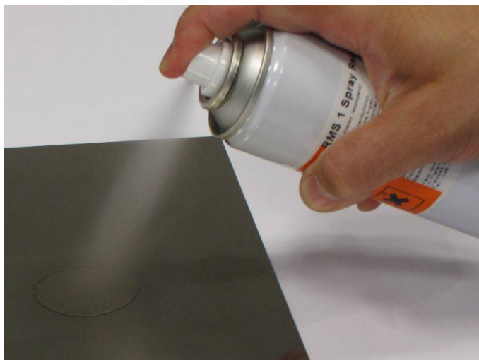
Fig. 2.1 Spraying 1-RMS on specimen
