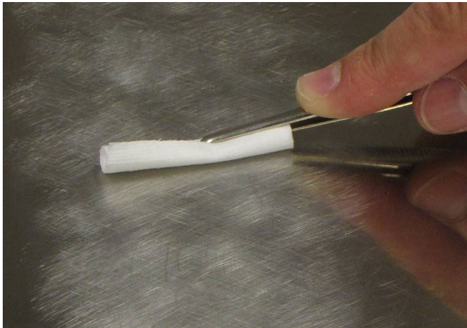
Fig. 2.4 Cleaning the roughened installation surface
