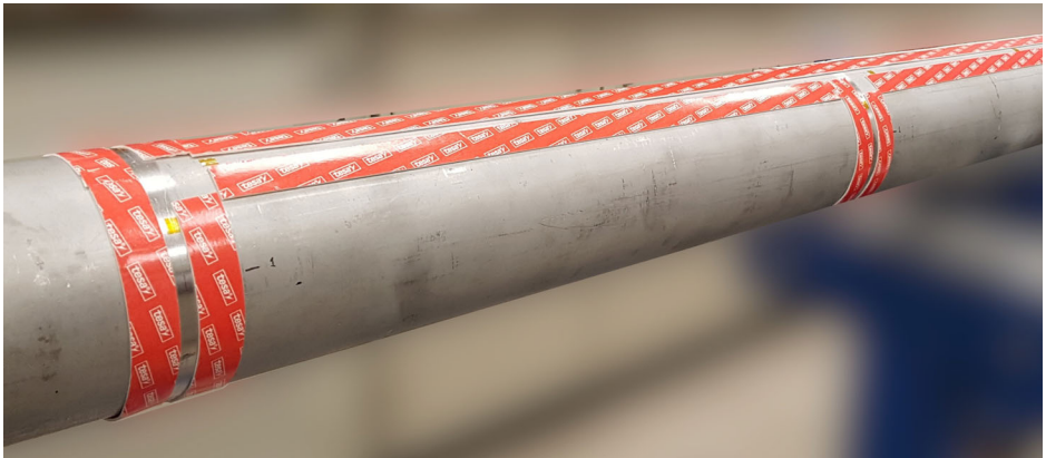
Fig. 2.20 Groove along the fiber using foam tape (optional).
