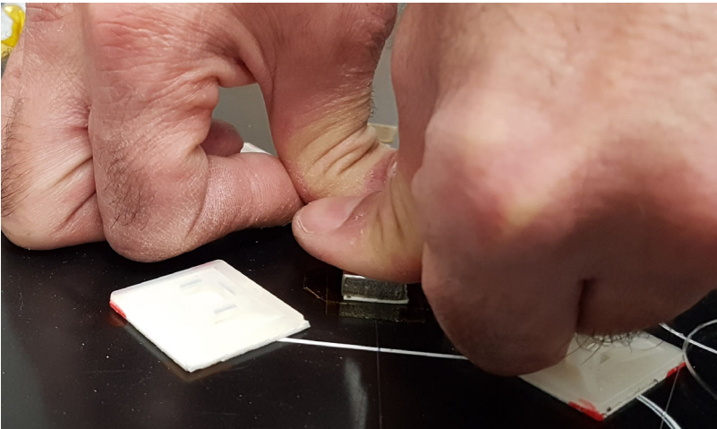
Fig. 2.19 Applying uniform pressure over the FBG.
