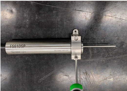
Fig. 2.5 Fixing the sensor brackets
