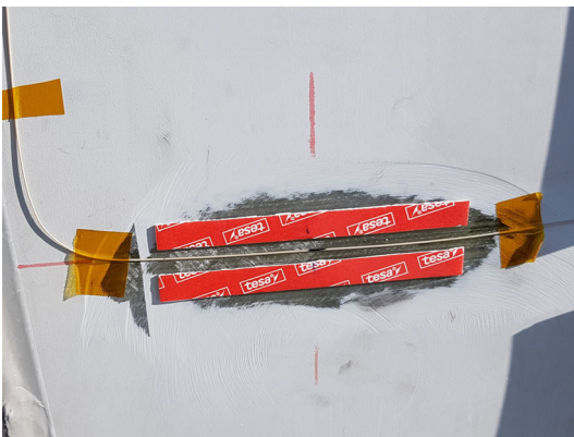
Fig. 2.8 Gluing frame created using foam tape (optional).
