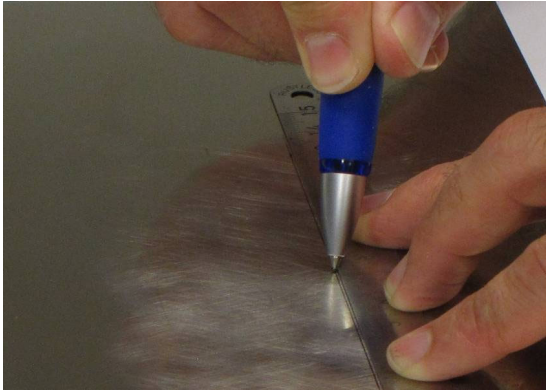
Fig. 2.6 Marking the marking lines
