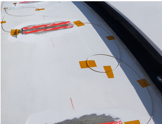
Fig. 2.18 Coiling the extra fiber length.
