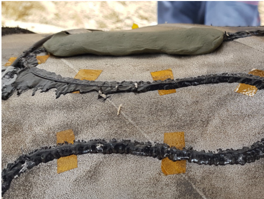
Fig. 2.16 Protecting the sensor with AK22.
