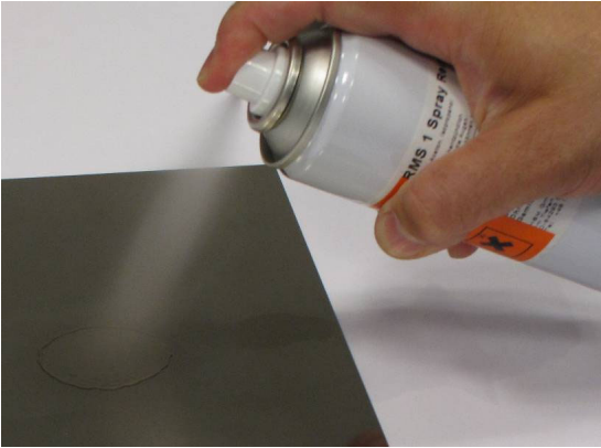
Fig. 2.1 Spraying the measuring point with 1-RMS-SPRAY
