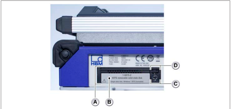
Fig. 7.4 GEN7iB removable drive bay
