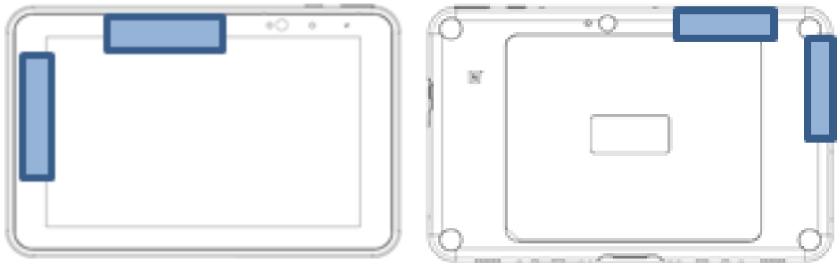
Fig. 1.1 Position of antennas
