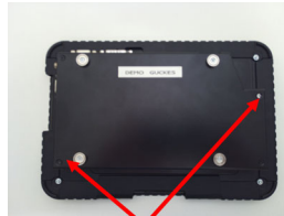
2 sealed screws to detect unauthorized opening
