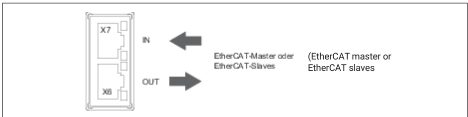
Fig. 9.2 X6, X7: Pin assignment for EtherCAT
