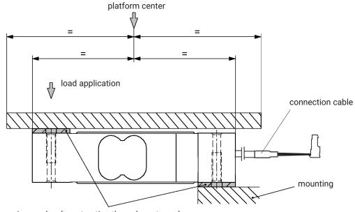
spacing washer (construction through customer)
