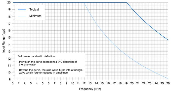
Note: Plot shows full power bandwidth for an overall gain of 0.2 or a 20  $V_{pp}$  input range. For other gain settings, scale the input range by the appropriate value. For example, for an overall gain of 0.05, multiply the 20  $V_{pp}$  scale by 4 for a 80  $V_{pp}$  input range.
