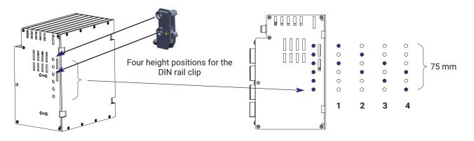
Basic device, WGX001/WGX002 for max. 5 plug-in cards
