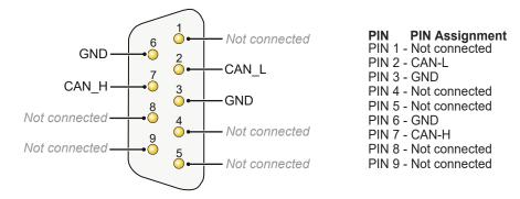
Figure 1.28: Pin assignment D-Sub
