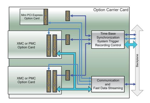
Figure 1.21: Block diagram option carrier card
