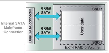
Figure 1.20: Block diagram drive
