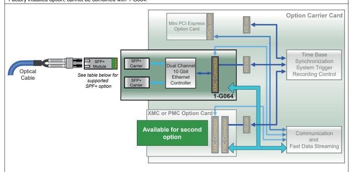
Figure 1.22: Block diagram 10Gbit Ethernet card, optical (G081 required)
