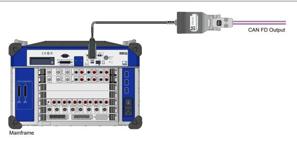
Figure 1.27: GEN7tA stand-alone CAN FD output
