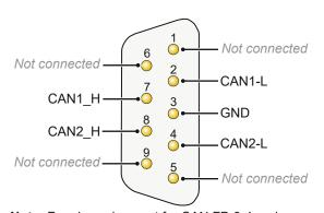
Note: For pin assignment for CAN FD 3-4 replace CAN1 with CAN3 and CAN2 with CAN4
