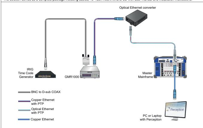
Figure 1.34: Example setup IRIG time synchronization
