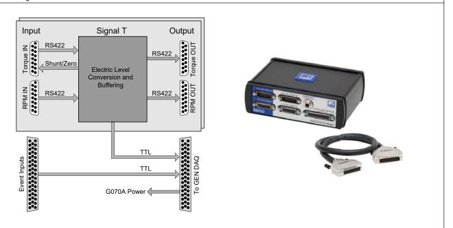
Figure 1.32: Block diagram and image
