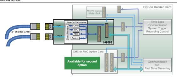
Figure 1.24: Block diagram EtherCAT® card
