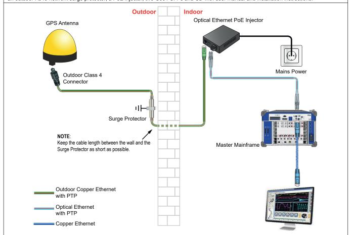
Figure 1.35: Example setup GPS time synchronization
