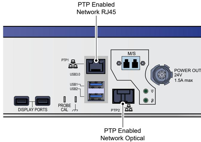
**Figure 1.8:** Electrical and optical 1 Gbit network interface
