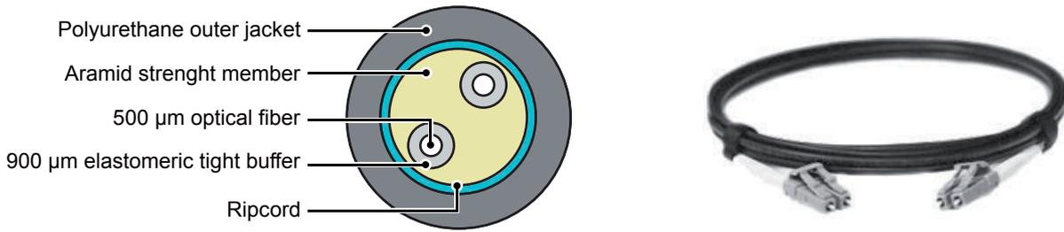
**Figure 1.32:** Block diagram and image
