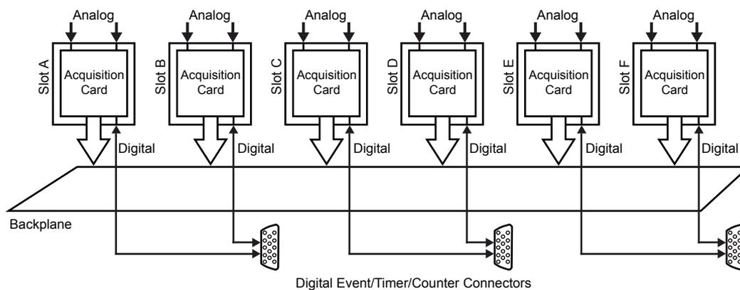
**Figure 1.14:** Digital Event/Timer/Counter block diagram
