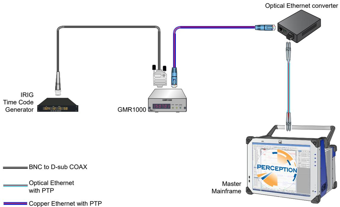
**Figure 1.35:** Example setup IRIG time synchronization
