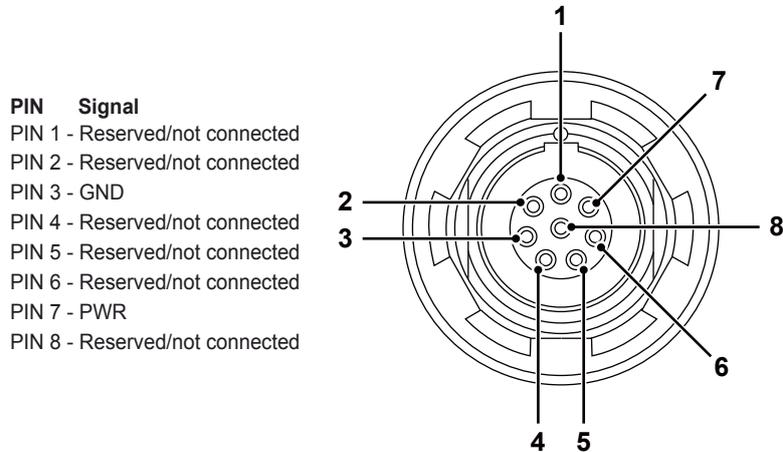
Figure 1.17: Connector power output
