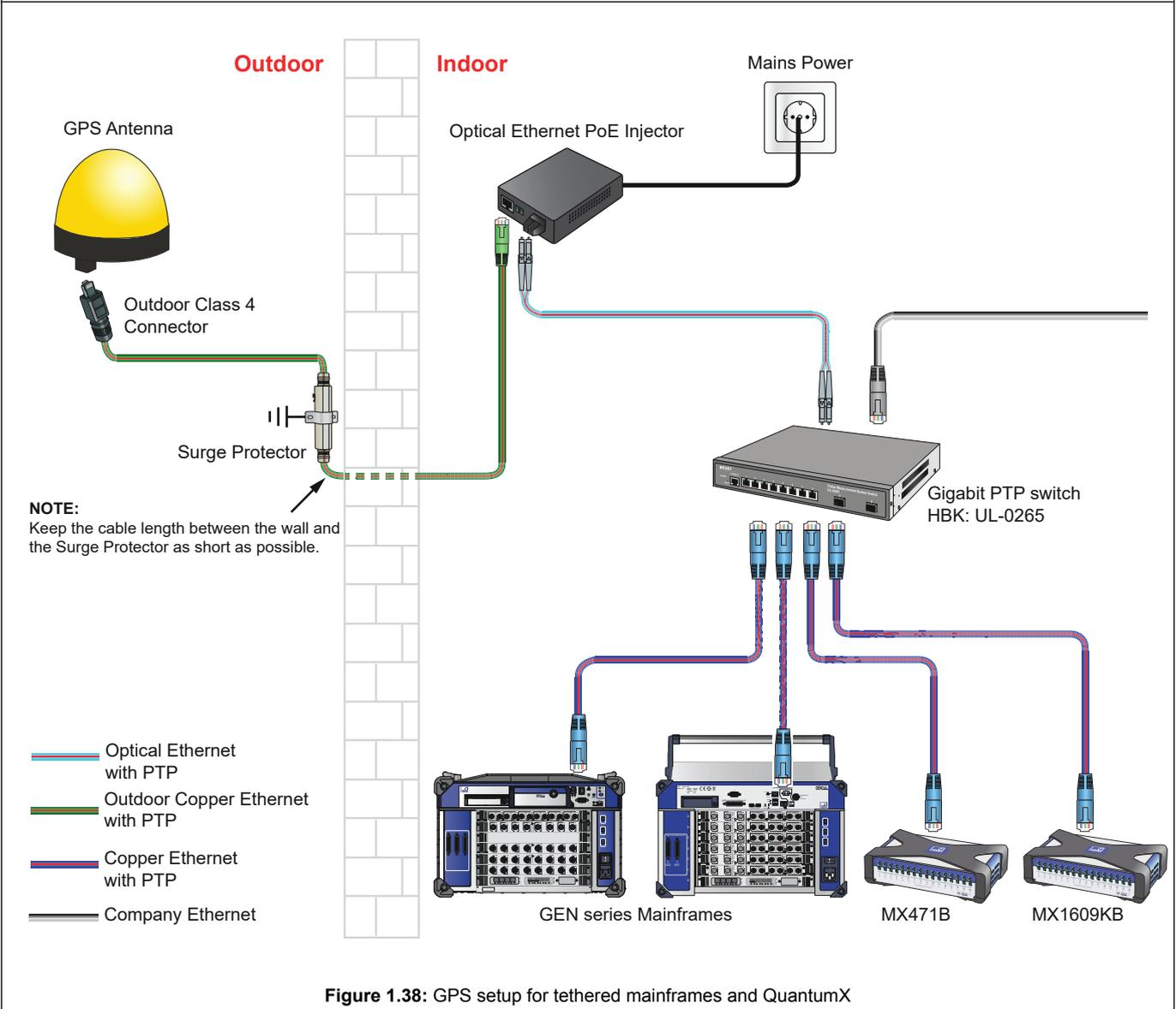
**Figure 1.38:** GPS setup for tethered mainframes and QuantumX
