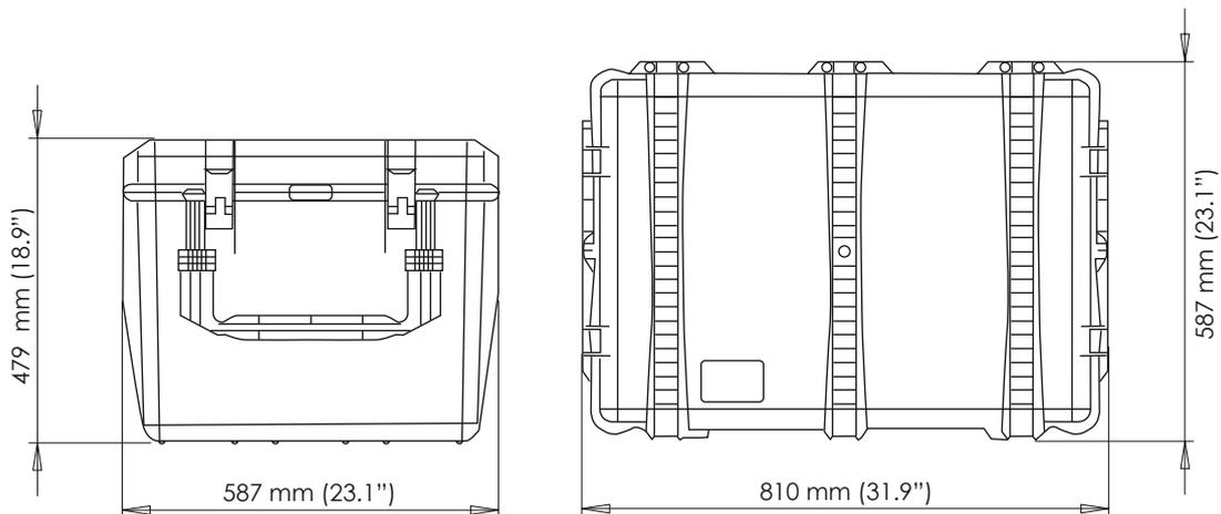
**Figure 1.40:** Reusable hardcover shipping case with wheels and transport handle
