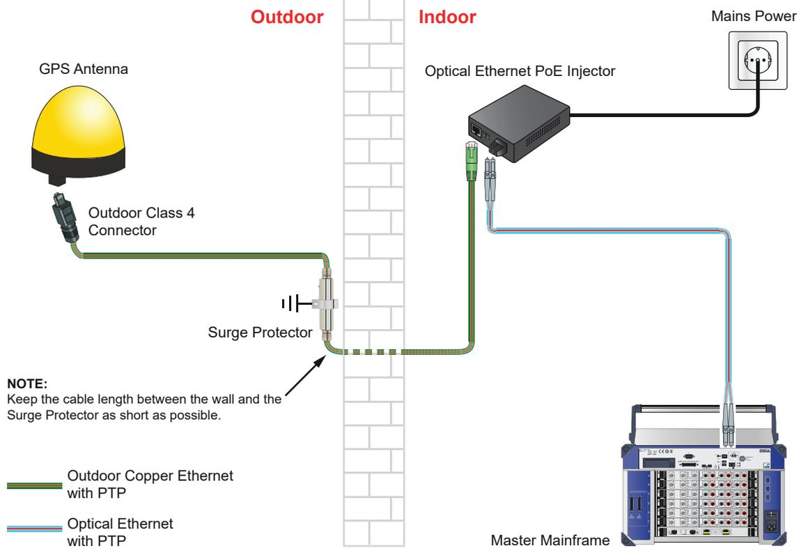
**Figure 1.36:** Example setup GPS time synchronization
