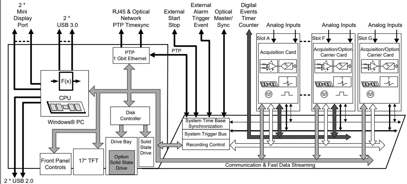
Figure 1.6: Block diagram
