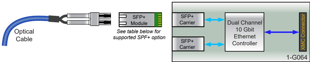
**Figure 1.26:** Block diagram 10Gbit Ethernet card, optical (G081 required)
