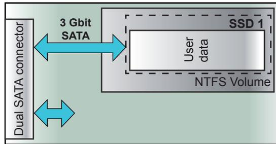
**Figure 1.23:** Block diagram removable Solid State Drive
