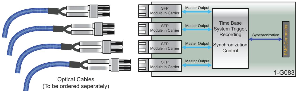
Figure 1.25: Block diagram Master output card (G081 required)
