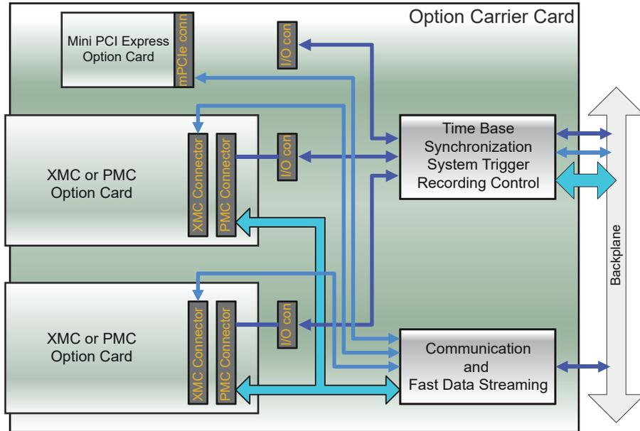
**Figure 1.24:** Block diagram option carrier card
