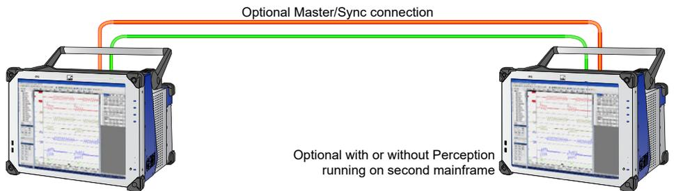
Figure 1.3: Dual mainframe
