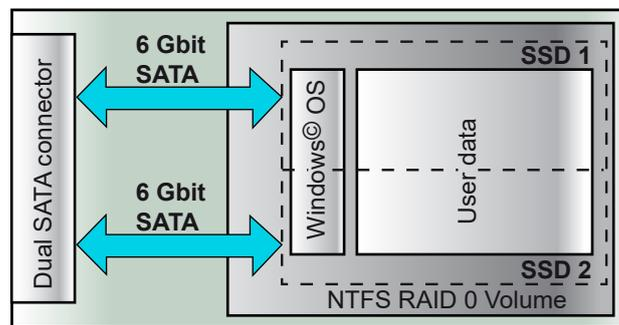
**Figure 1.21:** Block diagram removable system Solid State Drive
