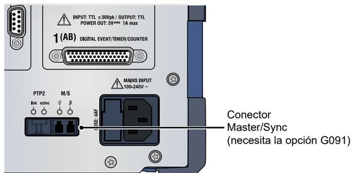
**Figura 12:** Conector Master/Synch
