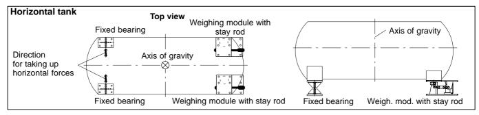
\* The application examples shown here are not suitable for use in all installing conditions. In each case the static, dynamic and thermal loads must be checked and the arrangement must be adjusted accordingly.
