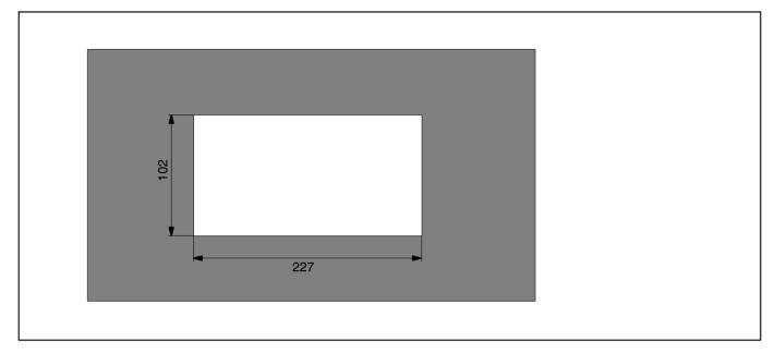
**Dimensions (desktop housing, also for wall mounting);** (in mm; 1 mm= 0.03937 inches)
