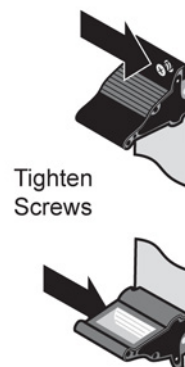
Figure 7.8: Card/module ejectors with screws
