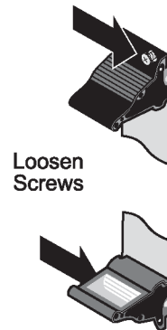
Figure 7.4: Card/module ejectors with screws
