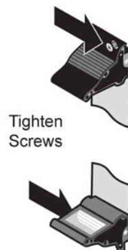
Figure 7.4: Card/module ejectors with screws
