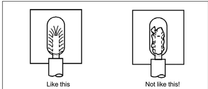
Fig. 4.7 Solder edges
