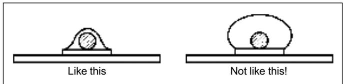
*Fig. 4.6 Soldered spot in cross-section*
