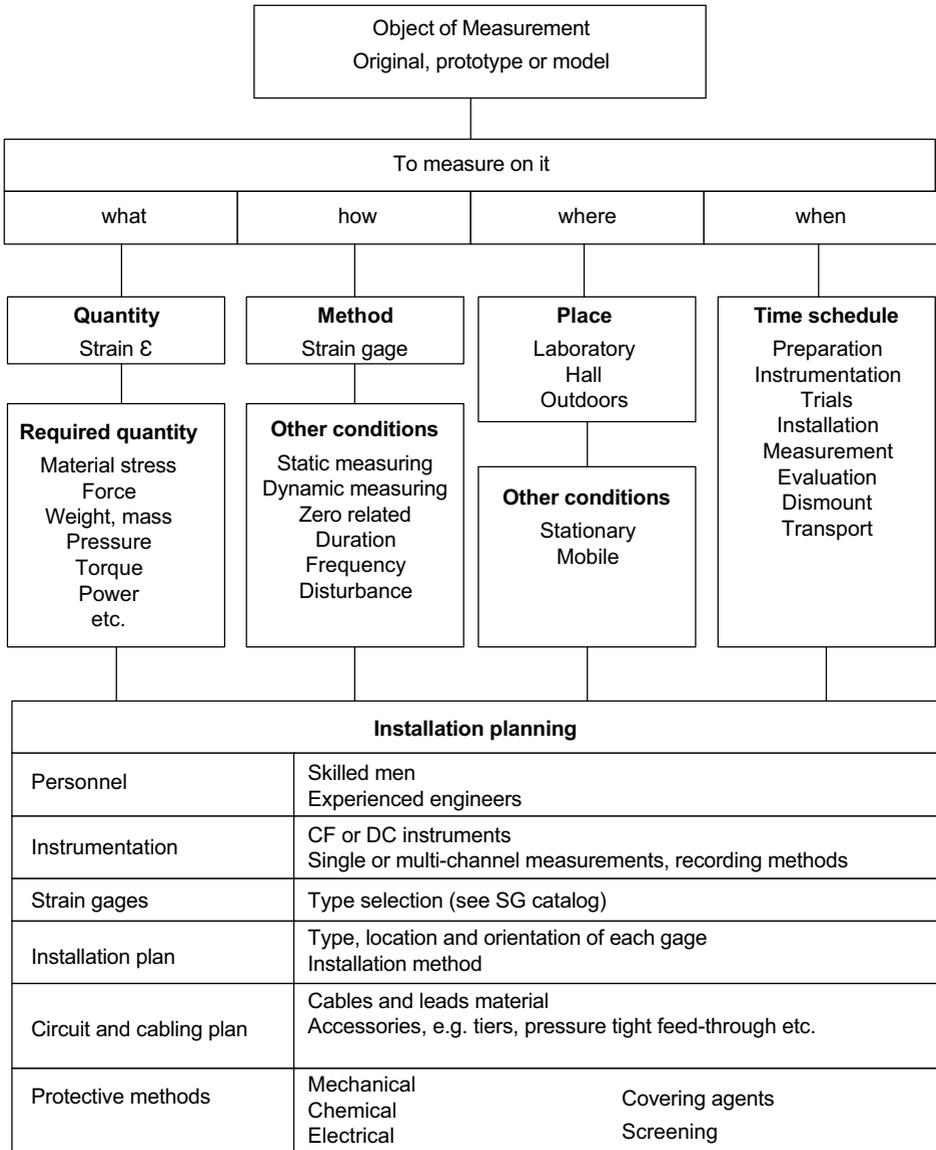
Fig. 2.1 Schematic of installation planning.
