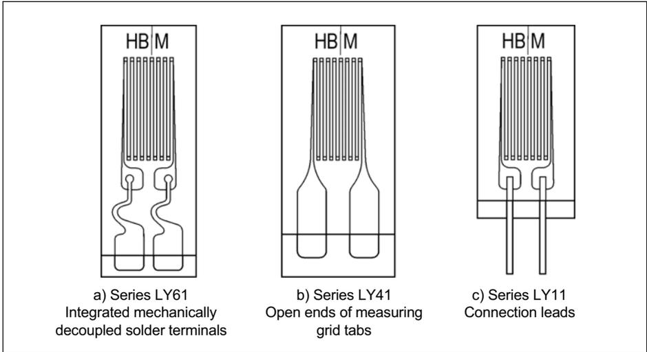
Fig. 3.4 Types of SG connections
