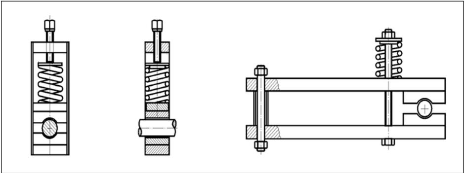
Fig. 3.9 Examples of spring-loaded clamps for SG installation with hot curing adhesives
