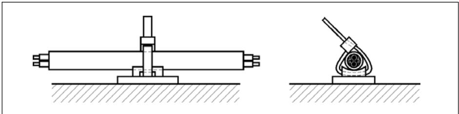
Fig. 4.9 Cable fixing with cable clips
