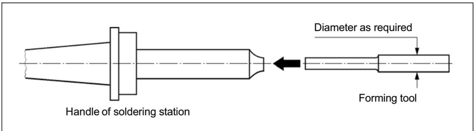
Fig. 3.2 Auxiliary tool for forming SG to fit small radii (only necessary for phenolic resin carrier SG)
