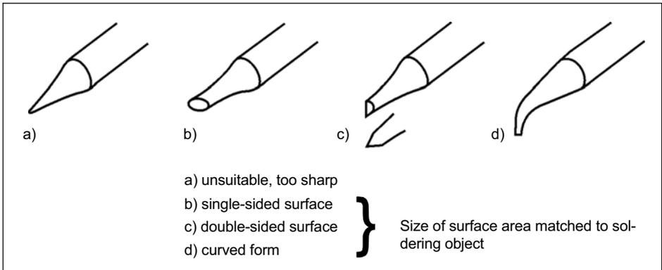
*Fig. 4.1 Various soldering tip shapes*
