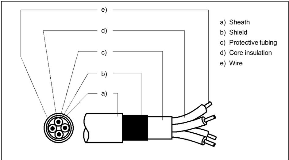
Fig. 4.3 Structure of a 4-wire HBM measuring cable
