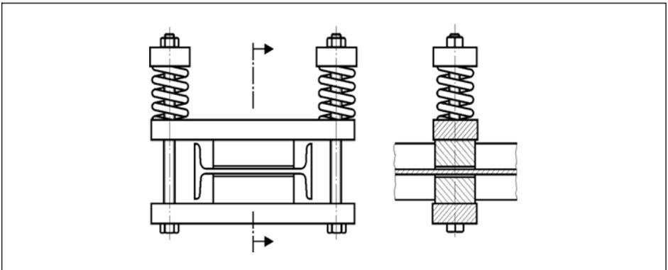
Fig. 3.10 Examples of spring-loaded clamps for SG installation with hot curing adhesives
