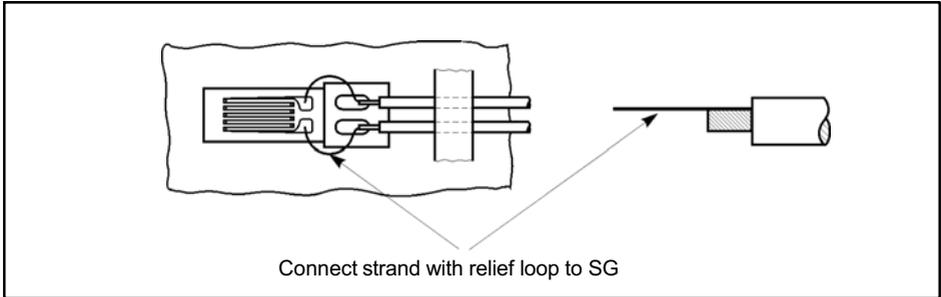
*Fig. 4.5 Connecting cable wires onto SG with open solder tabs*
