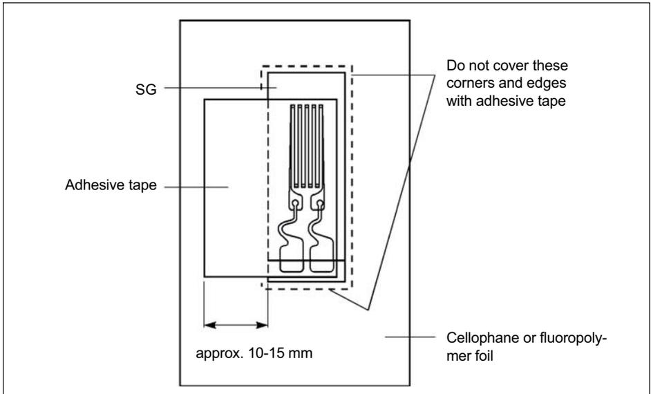
*Fig. 3.5 Auxiliary technique 1 for SG installation*
