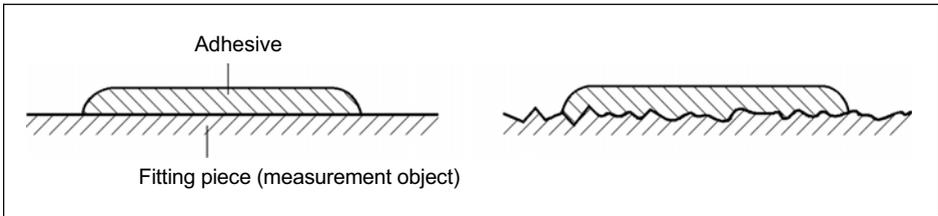
*Fig. 3.1 Influence of surface roughness on effective contact surface size*
