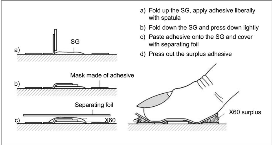
Fig. 3.8 Installing strain gages with superglue X60
