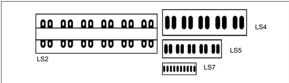
*Fig. 4.2 Some solder terminal forms (examples)*
