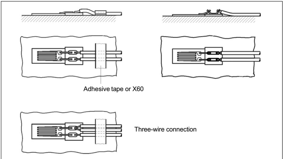
Fig. 4.4 Soldering cable wires onto SG with connection leads
