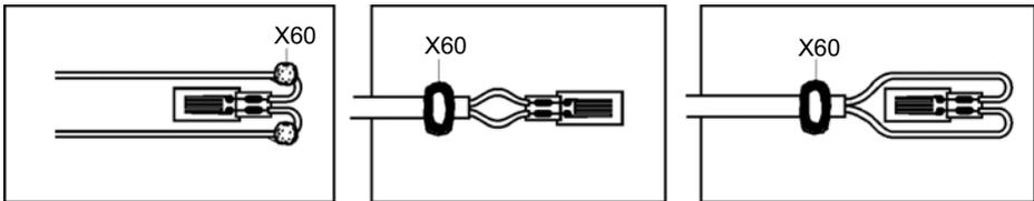
Fig. 4.10 Various options for cable fixing with X60
