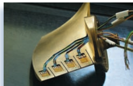
Testing of a turbine wing under laboratory conditions
