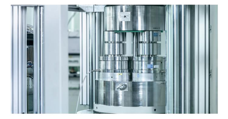
FORM + TEST as prescribed by PTB. A DAkkS calibration of the BU18 had been performed in HBK's accredited calibration laboratory in advance. Traceability of the calibration to the National Standard (PTB) has, therefore, been ensured.
