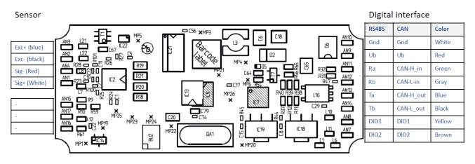
The AD112D must always be connected to a power supply via the **GND** and **Ub** pins and is therefore not supplied via the adapter.
