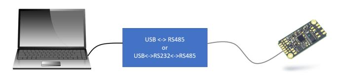
After that the software PanelX by HBM can be used to configure the transducer electronic.
