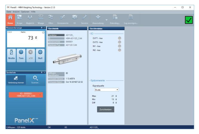
In the upper region are several menus that lead to configuration content of AD112D. For example, the adjustment can be performed.
