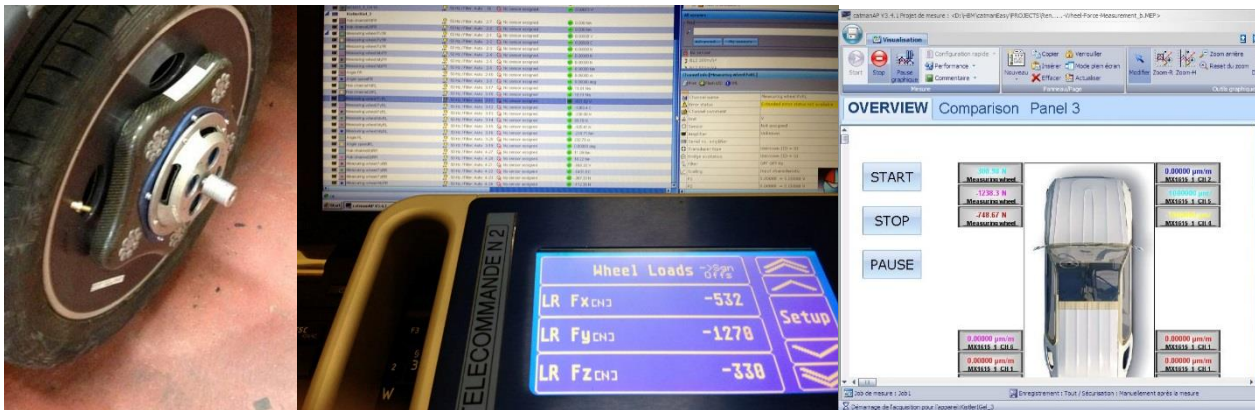
Picture: Kistler wheel, remote control and screenshot showing live data acquired over Ethernet
