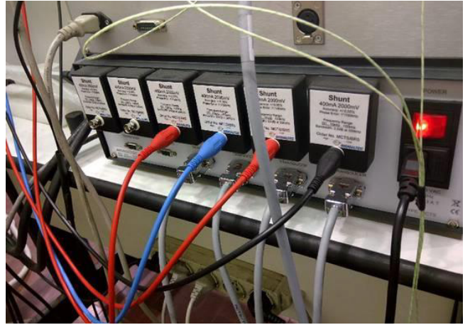
Fig. 3.b: Rear of the current sensors box
