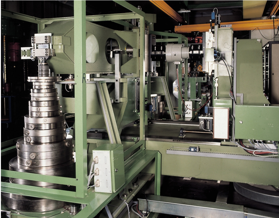
Fig. 7.1 Calibration machine based on the lever-arm-mass principle
