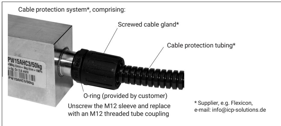
Even without a cable protection system, standard load cells can achieve an IP rating of IP68/IP69K. In applications where the PVC cable of the load cell could be chemically or mechanically attacked or destroyed, extra cable protection can be provided using standard cable protection systems.
