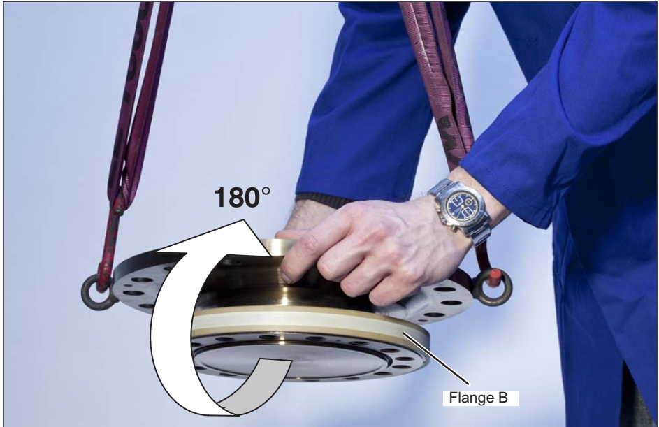
Fig. 5.2 Rotating the rotor
