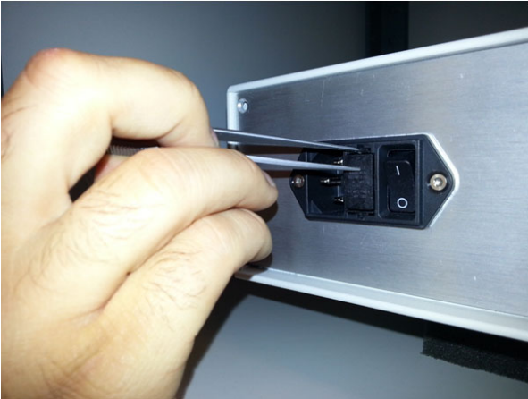
Fig. 4.12 Removing the fuse
