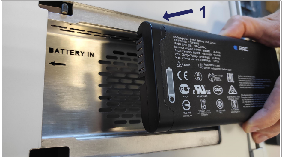
Fig. 3.10 Aligning the battery pack
