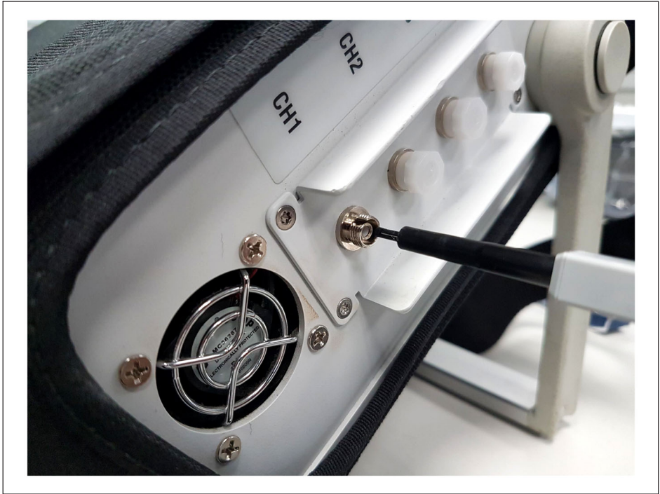
Fig. 4.7 Cleaning the adapter
