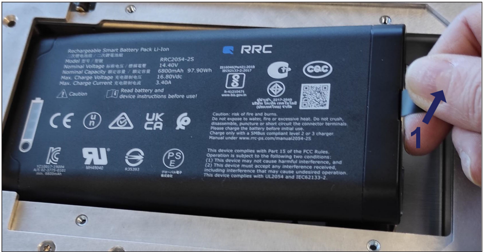
Fig. 3.9 Removing the battery pack
