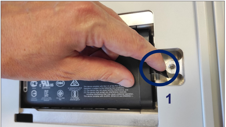
Fig. 3.11 Positioning the pull-out flap
