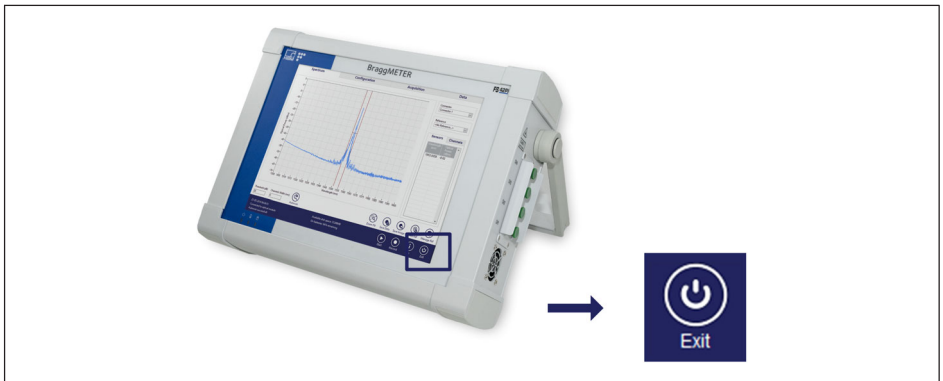
Fig. 3.3 Switching off via software
