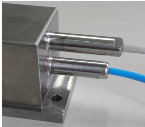
The hose and the plug should only be removed once it is certain that the atmosphere is not potentially explosive, or if the electrical equipment inside the housing has been disconnected from the mains for at least five minutes and is voltage-free.
