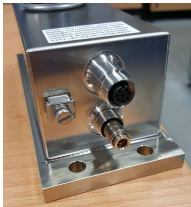
The quick-release coupling is closed without its counterpart. When a hose is connected, this must finish with its open end outside zone 22 (no potentially explosive atmosphere). Secure protection must be provided to prevent the ingress of dust and moisture.
