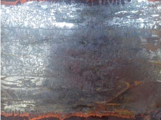
Fig. 2.2 Uneven and rusty surface unsuited for welding sensor
