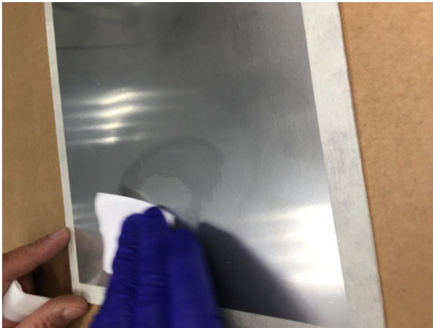
Fig. 2.6 Cleaning the surface
