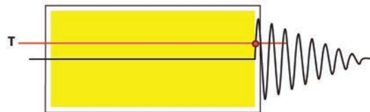
Figure 9.6: Full pre-trigger storage: pre-trigger = 100%
