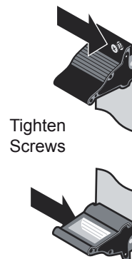
Figure 7.5: Card ejectors with screws
