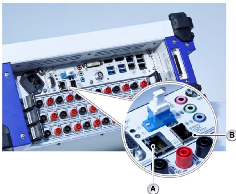
Figure F.6: GEN3i PTP enabled ports
