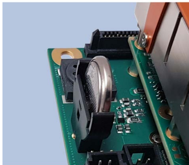
Figure 4.2: Battery - PC section
