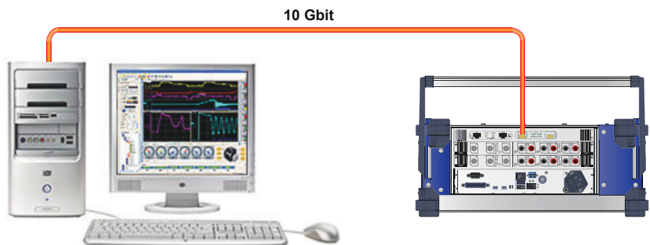
Figure 11.18: Basic setup - 10 Gbit Ethernet to PC
