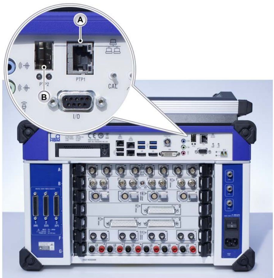
Figure F.1: GEN7i PTP enabled ports
