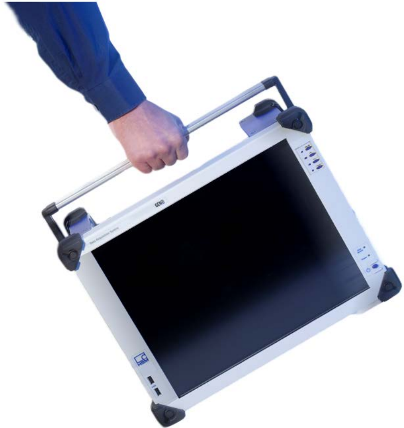
Figure 7.7: GEN3iA with handle in the upright position
