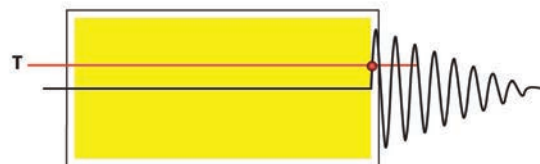
Figure 9.6: Full pre-trigger storage: pre-trigger = 100%
