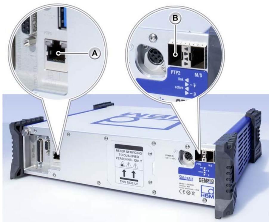
Figure F.4: GEN2tB PTP enabled ports
