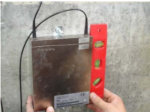
Fig. 2.6 Vertical alignment using a bubble level
