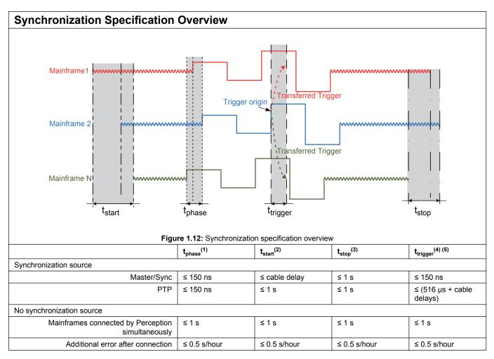
(1) t<sub>phase</sub> Maximum phase difference between signals. (*This specification is not affected by any of the other specifications*).
