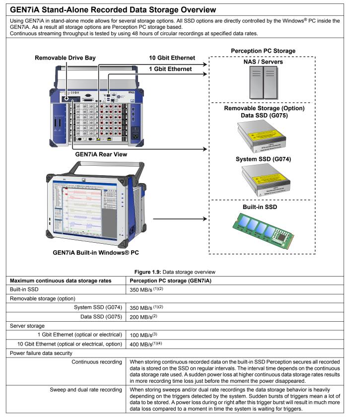
(1) Legacy cards do not support the enhanced fast streaming bus. The maximum aggregate storage rate for legacy cards is 200 MB/s.
