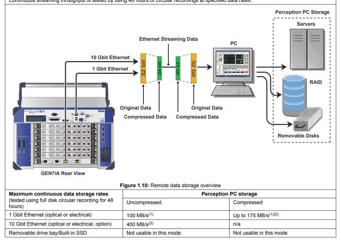
(1) Test setup uses a Windows® PC with Intel i7 CPU and SSD with sustained write speeds exceeding 250 MB/s.
