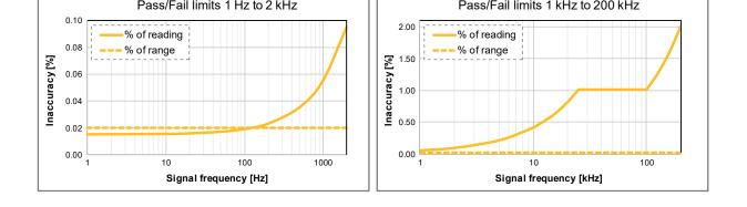
**Figure 4:** Power pass/fail limits (0.33  $\Omega$  shunt), Wideband and 0.5  $\leq$  Power Factor  $\leq$  1
